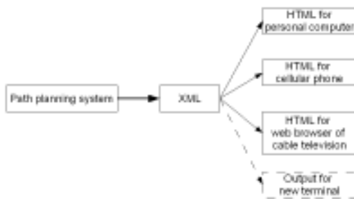
Fig. 3. Relation among path planning system, intermediate output, and output form of each device.
